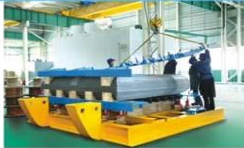
大型变压器铁芯翻砂台 Large flip bench of transformer core
